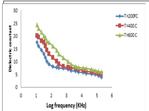
Fig (3) Dielectric constant as a function of frequency
