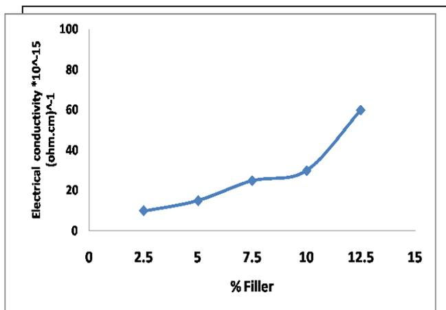
Fig (6) Electrical conductivity as a function of weight fraction
