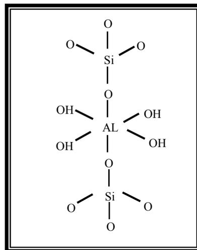
Figure(1) Diagram for bentonite structure <sup>(7)</sup>
