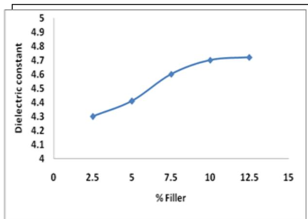
Fig (7) Dielectric constant as a function of weight fraction
