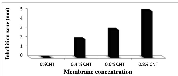
Figure (9): Effect of MWCNT /Nylon ratio in inhibition zone against (*E.coli.*) bacteria.
