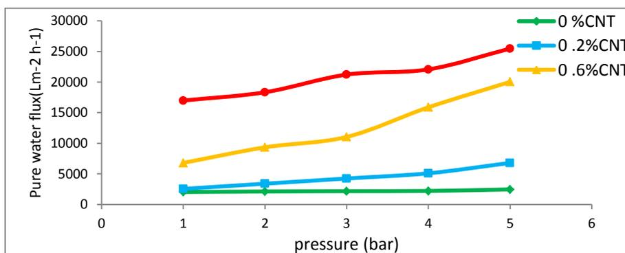
Figure (6): Effect of membrane pressure on the pure water permeation flux of the Nylon 6/MWCNT nanofiber membrane at room temperature and 50 min time.
