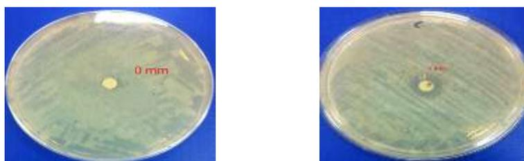
Figure (8): Shows the formation inhibition zone around the MWCNT/Nylon membrane, after 24 hrs. and 37°C.
