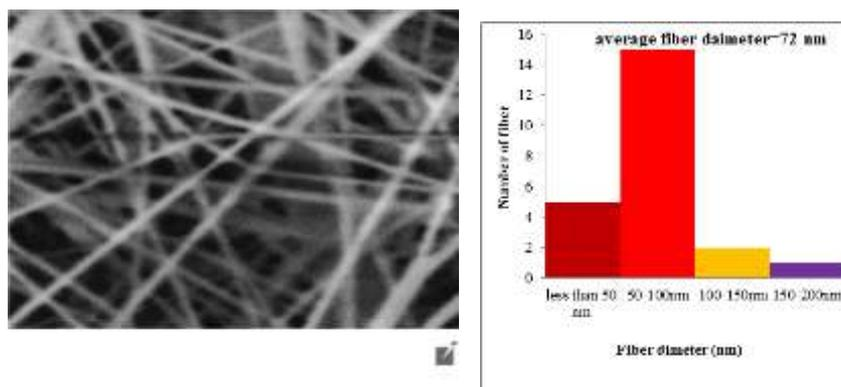
Figure (3): (a) SEM image of 0.8 wt. % MWCNT/ Nylon 6 nanofibers membrane, (b) fiber diameter distribution.
