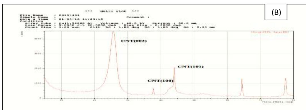
Figure (1): X-ray of (A) raw carbon nanotube, (B) acidic modification carbon nanotube by ((1/3) HNO<sub>3</sub>/H<sub>2</sub>SO<sub>4</sub>).
