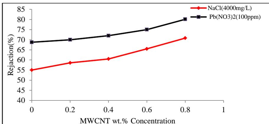
Figure (7): Effect of MWCNT/Nylon 6 ratio on rejection of  $Pb(NO_3)_2$  salt and NaCl salt aqueous solutions with initial concentration 100 ppm and 4000mg/L respectively, at room temperature and 1 bar.
