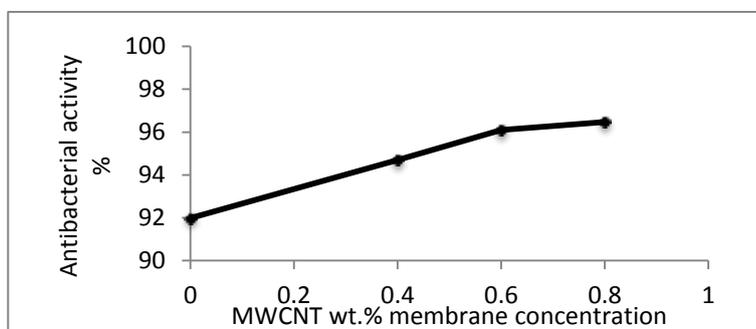
Figure (10): Effect of MWCNT addition in the antibacterial activity at room temperature.
