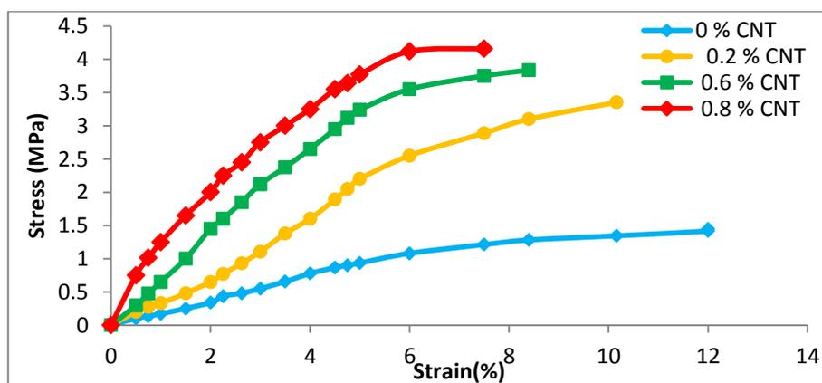
Figure (12): Stress – Strain curve of MWCNT /Nylon 6 with various ratios.
