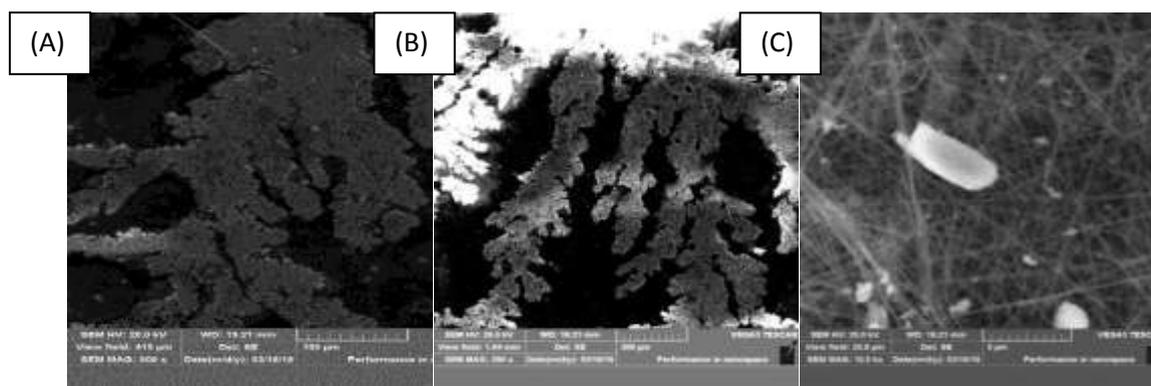
Figure (11): SEM of membrane after exposing to bacteria, where the bacteria cluster: (A) on the membrane surface as a dendritic shape colony, (B) and (C) shows how fiber capture the bacteria.
