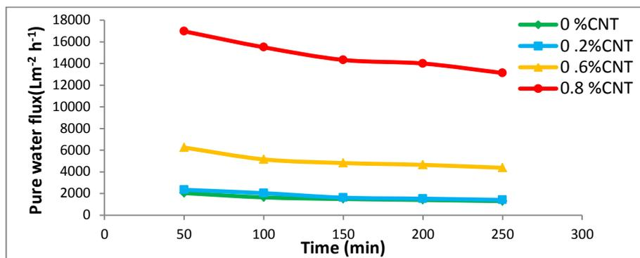
Figure (5): Pure water permeation flux with time of Nylon 6 /MWCNT nanofiber membrane at room temperature and (1 bar) pressure.
