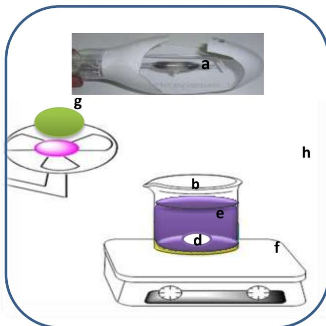
Scheme1. Schematic diagram of photo-reactor components. Whereas, a) (250 W) High pressure mercury lamp,(b) 400 cm<sup>3</sup> Pyrex glass beaker, (c) dispersive blue 26 dye with ZnO as suspension solution, (d)Teflon bar, (e)suspension solution (Dye with photo-catalyst), (f) magnetic stirrer, (g) fan and (h) wooden box.
