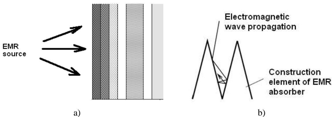
Figure 1 - Examples of structures of EMR absorbers
