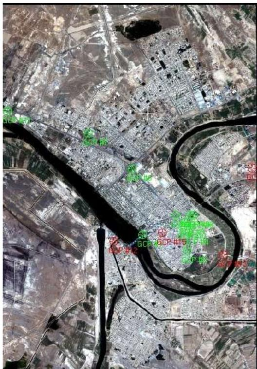
Figure (4): The location of GCPs & check points for high resolution
