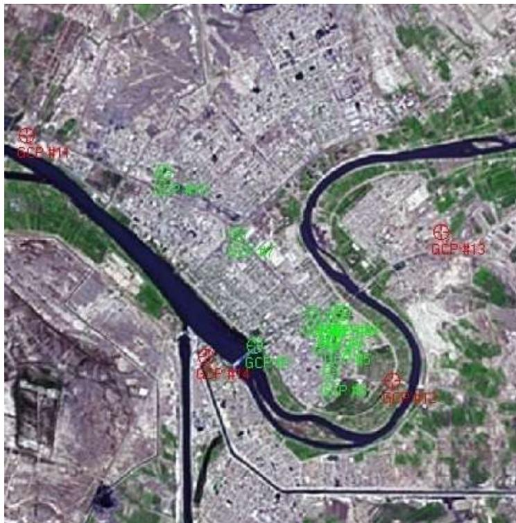
Figure (5): The location of GCPs & check points for low resolution image.
