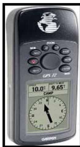
**Figure (3): Garmin GNSS 72 GNSS Device.**
