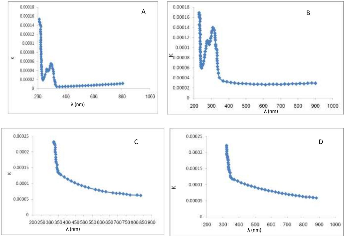
Fig.4. Extinction coefficient as a function wavelength for A-Pure PMMA polymer, B- 0.01% , C-0.03%, D- 0.05% polymer doped ITO
