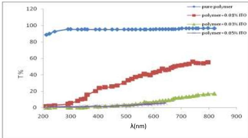
Fig.1. Transmission spectrum for pure and doped polymer
