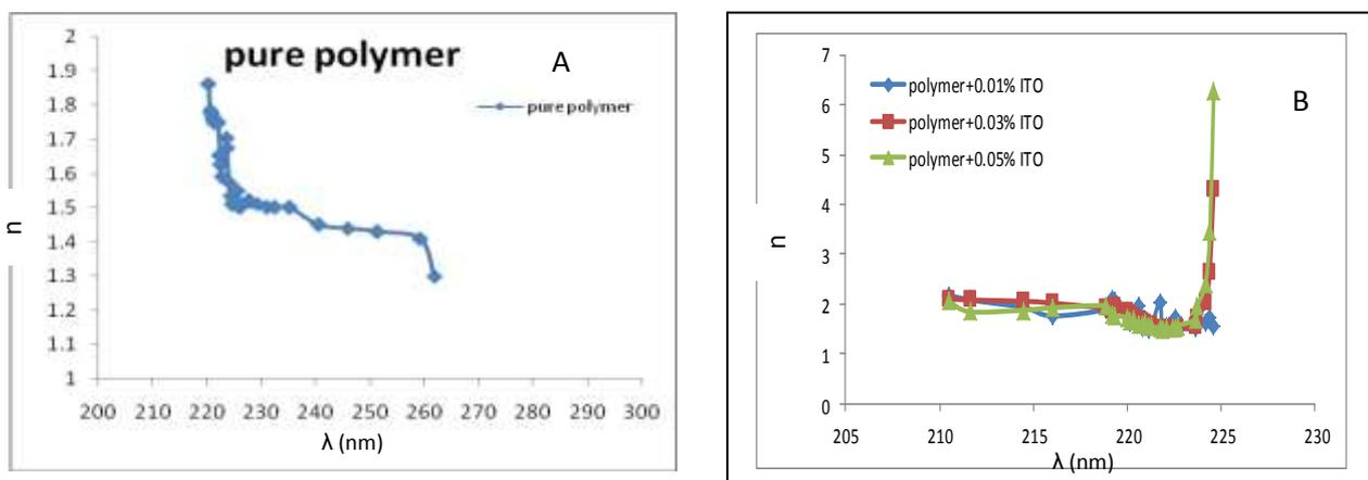
Fig. 5. Refractive index vs. wave length ( $\lambda$ ) plots for A- Pure polymer, B- doped polymer composites.
