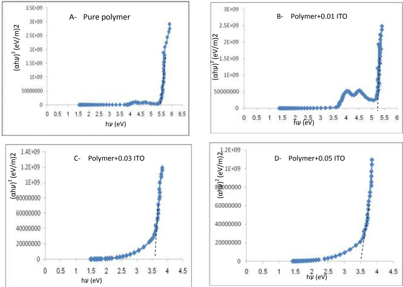
Fig.3.  $(\alpha h\nu)^2$  vs.  $h\nu$  plots of PMMA-ITO composites. A-pure polymer, B- 0.01% , C-0.03%, D- 0.05% polymer doped ITO
