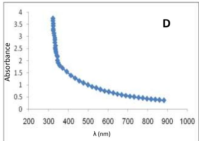
Fig.2. The absorption spectrum of of PMMA-ITO composites. A-pure polymer, B- 0.01% , C- 0.03%, D- 0.05% polymer doped ITO
