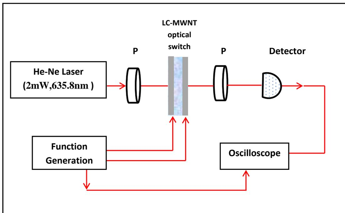
Fig.(2) Experimental setup for measuring the electro-optical properties of the LCD devices with an applied AC voltage
