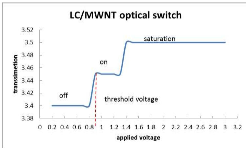
Fig.(3) Threshold voltage of LC/MWNT optical switch
